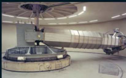
This centrifuge is designed to test the effects of linear acceleration on visual function in space
